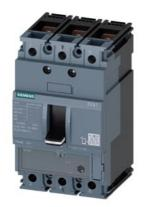
circuit breaker 3VA1 IEC Frame 160 breaking capacity class M Icu=55 kA @ 415 V 3-pole, starter protection TM120M, AM, In=20 A without overload protection short-circuit protection Ii=7...16 x In nut keeper kit
