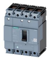
circuit breaker 3VM1 IEC frame 160 breaking capacity class N Icu=25kA @ 415V 4-pole, line protection TM220, ATFM, In=100A overload protection Ir=70A...100A short-circuit protection Ii=10 x In N conductor protection 100% nut keeper kit
