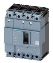
circuit breaker 3VM1 IEC frame 160 breaking capacity class S Icu=36kA @ 415V 4-pole, line protection TM220, ATFM, In=20A overload protection Ir=14A ...20A short-circuit protection Ii=16 x In N conductor protection nut keeper kit
