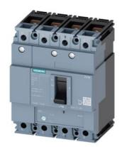
circuit breaker 3VM1 IEC frame 160 breaking capacity class S Icu=36kA @ 415V 4-pole, line protection TM220, ATFM, In=63A overload protection Ir=44A...63A short-circuit protection Ii=10 x In N conductor protection 100% nut keeper kit
