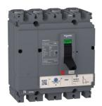
circuit breaker EasyPact CVS160B, 25 kA at 415 VAC, 160 A rating thermal magnetic TM-D trip unit, 4P 3d
