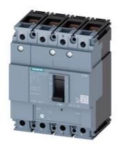
circuit breaker 3VM1 IEC frame 160 breaking capacity class M Icu=55kA @ 415V 4-pole, line protection TM220, ATFM, In=20A overload protection Ir=14A...20A short-circuit protection Ii=16 x In N conductor protection 100% nut keeper kit
