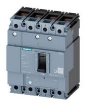
circuit breaker 3VM1 IEC frame 160 breaking capacity class M Icu=55kA @ 415V 4-pole, line protection TM220, ATFM, In=50A overload protection Ir=35A...50A short-circuit protection Ii=10 x In N conductor protection 100% nut keeper kit
