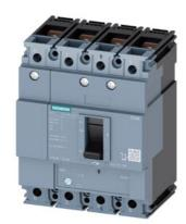
circuit breaker 3VM1 IEC frame 160 breaking capacity class M Icu=55kA @ 415V 4-pole, line protection TM220, ATFM, In=16A overload protection Ir=11A...16A short-circuit protection Ii=20 x In N conductor protection 100% nut keeper kit
