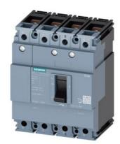
circuit breaker 3VM1 IEC frame 160 breaking capacity class N Icu=25kA @ 415V 4-pole, line protection TM210, FTFM, In=160A overload protection Ir=160A, not adjustable short-circuit protection Ii=10 x In N conductor unprotected nut keeper kit
