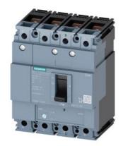
circuit breaker 3VM1 IEC frame 160 breaking capacity class N Icu=25kA @ 415V 4-pole, line protection TM220, ATFM, In=160A overload protection Ir=112A...160A short-circuit protection Ii=10 x In N conductor protection 100% nut keeper kit
