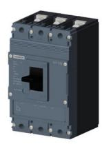
circuit breaker 3VJ1 IEC framesize 3VJ11 125A line protection FTFM 3-pole Icu=36kA@415V Ics=75% Icu In=20A overload protection Ir=20A short-circuit protection Ii=450A Screw connection
