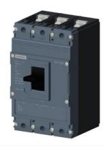
circuit breaker 3VJ1 IEC framesize 3VJ11 125A line protection FTFM 3-pole lcu=36kA@415V lcs=75% lcu ln=80A overload protection lr=80A short-circuit protection li=10 x ln Screw connection
