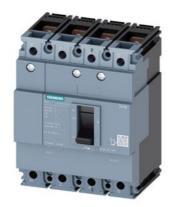
circuit breaker 3VM1 IEC frame 160 breaking capacity class S Icu=36kA @ 415V 4-pole, line protection TM210, FTFM, In=125A overload protection Ir=125A, not adjustable short-circuit protection Ii=10 x In N conductor protection 100% nut keeper kit
