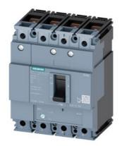
circuit breaker 3VM1 IEC frame 160 breaking capacity class S Icu=36kA @ 415V 4-pole, line protection TM220, ATFM, In=160A overload protection Ir=112A...160A short-circuit protection Ii=10 x In N conductor protection 100% nut keeper kit
