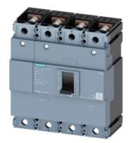
circuit breaker 3VM1 IEC frame 250 breaking capacity class S Icu=36kA @ 415V 4-pole, line protection TM210, FTFM, In=200A overload protection Ir=200A, not adjustable short-circuit protection Ii=10 x In N conductor protection 100% nut keeper kit
