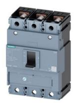
circuit breaker 3VM1 IEC frame 250 breaking capacity class S Icu=36kA @ 415V 3-pole, line protection TM220, ATFM, In=200A overload protection Ir=140A...200A short-circuit protection Ii=10 x In nut keeper kit
