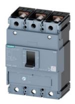
circuit breaker 3VM1 IEC frame 250 breaking capacity class M Icu=55kA @ 415V 3-pole, line protection TM220, ATFM, In=200A overload protection Ir=140A...200A short-circuit protection Ii=10 x In nut keeper kit
