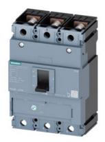
circuit breaker 3VM1 IEC frame 250 breaking capacity class S Icu=36kA @ 415V 3-pole, line protection TM220, ATFM, In=250A overload protection Ir=175A...250A short-circuit protection Ii=10 x In nut keeper kit
