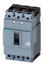
circuit breaker 3VM1 IEC frame 100 breaking capacity class N Icu=25kA @ 415V 3-pole, line protection TM210, FTFM, In=63A overload protection Ir=63A, not adjustable short-circuit protection Ii=10 x In nut keeper kit
