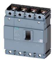
circuit breaker 3VM1 IEC frame 250 breaking capacity class S Icu=36kA @ 415V 4-pole, line protection TM210, FTFM, In=250A overload protection Ir=250A, not adjustable short-circuit protection Ii=10 x In N conductor protection 100% nut keeper kit
