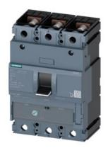
circuit breaker 3VA1 IEC Frame 250 breaking capacity class H Icu=70 kA @ 415 V 3-pole, line protection TM220, ATFM, In=200 A overload protection Ir=140 A...200 A short-circuit protection Ii=10 x In nut keeper kit
