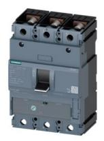
circuit breaker 3VA1 IEC Frame 250 breaking capacity class H Icu=70 kA @ 415 V 3-pole, line protection TM220, ATFM, In=250 A overload protection Ir=175 A...250 A short-circuit protection Ii=10 x In nut keeper kit
