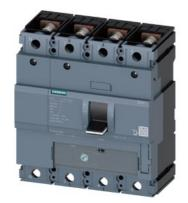
circuit breaker 3VA1 IEC Frame 250 breaking capacity class H Icu=70 kA @ 415 V 4-pole, line protection TM220, ATFM, In=250 A overload protection Ir=175 A...250 A short-circuit protection Ii=10 x In neutral conductor protection 100% nut keeper kit
