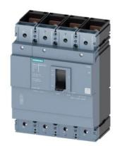
circuit breaker 3VM1 IEC frame 400 breaking capacity class N Icu=36kA @ 415V 4-pole, line protection TM210, FTFM, In=400A overload protection short-circuit protection Ii=10 x In N conductor protection 100% nut keeper kit
