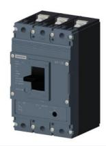
circuit breaker 3VJ1 IEC framesize 3VJ11 125A line protection ATFM 3-pole Icu=36kA@415V Ics=75% Icu In=40A overload protection Ir=32A...40A short-circuit protection Ii=600A Screw connection
