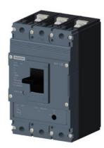
circuit breaker 3VJ1 IEC framesize 3VJ11 125A line protection ATFM 3-pole Icu=36kA@415V Ics=75% Icu In=50A overload protection Ir=40A...50A shortcircuit protection Ii=600A Screw connection
