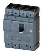
circuit breaker 3VA1 IEC Frame 630 breaking capacity class S Icu=36 kA @ 415 V 4-pole, line protection TM220, ATFM, In=500 A overload protection Ir=350 A...500 A short-circuit protection Ii=10 x In neutral conductor protection 100% nut keeper kit
