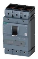
circuit breaker 3VA1 IEC Frame 630 breaking capacity class M Icu=55 kA @ 415 V 3-pole, starter protection TM120M, AM, In=500 A without overload protection short-circuit protection Ii=5...10 x In nut keeper kit
