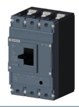
circuit breaker 3VJ1 IEC framesize 3VJ10 125A line protection ATFM 3-pole Icu=10kA@415V Ics=100% Icu In=16A overload protection Ir=12.8A..16A short-circuit protection Ii=500A Screw connection
