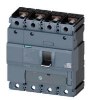
circuit breaker 3VA1 IEC Frame 250 breaking capacity class H Icu=70 kA @ 415 V 4-pole, line protection TM220, ATFM, In=200 A overload protection Ir=140 A...200 A short-circuit protection Ii=10 x In neutral conductor protection 100% nut keeper kit
