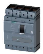
circuit breaker 3VA1 IEC Frame 400 breaking capacity class S Icu=36 kA @ 415 V 4-pole, line protection TM220, ATFM, In=400 A overload protection Ir=280 A...400 A short-circuit protection Ii=10 x In neutral conductor protection 100% nut keeper kit
