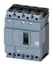
circuit breaker 3VM1 IEC frame 160 breaking capacity class N Icu=25kA @ 415V 4-pole, line protection TM220, ATFM, In=50A overload protection Ir=35A...50A short-circuit protection Ii=10 x In N conductor protection 100% nut keeper kit
