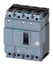
circuit breaker 3VM1 IEC frame 160 breaking capacity class N Icu=25kA @ 415V 4-pole, line protection TM220, ATFM, In=63A overload protection Ir=44A...63A short-circuit protection Ii=10 x In N conductor protection 100% nut keeper kit
