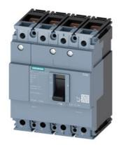
circuit breaker 3VM1 IEC frame 100 breaking capacity class B Icu=16kA @ 415V 4-pole, line protection TM210, FTFM, In=16A overload protection Ir=16A, not adjustable short-circuit protection Ii=20 x In N conductor unprotected nut keeper kit
