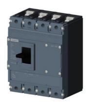
circuit breaker 3VJ1 IEC framesize 3VJ11 125A line protection FTFM 4-pole lcu=36kA@415V lcs=75% lcu In=20A overload protection Ir=20A short-circuit protection Ii=450A Screw connection
