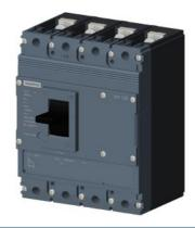
circuit breaker 3VJ1 IEC framesize 3VJ11 125A line protection FTFM 4-pole lcu=36kA@415V lcs=75% lcu ln=32A overload protection lr=32A short-circuit protection li=600A Screw connection
