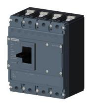
circuit breaker 3VJ1 IEC framesize 3VJ11 125A line protection FTFM 4-pole lcu=36kA@415V lcs=75% lcu ln=63A overload protection lr=63A short-circuit protection li=10 x ln Screw connection
