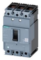
circuit breaker 3VM1 IEC frame 160 breaking capacity class N Icu=25kA @ 415V 3-pole, line protection TM220, ATFM, In=20A overload protection Ir=14A...20A short-circuit protection Ii=16 x In nut keeper kit
