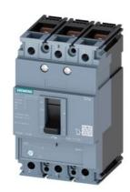
circuit breaker 3VM1 IEC frame 160 breaking capacity class N Icu=25kA @ 415V 3-pole, line protection TM220, ATFM, In=25A overload protection Ir=18A...25A short-circuit protection Ii=12.8 x In nut keeper kit
