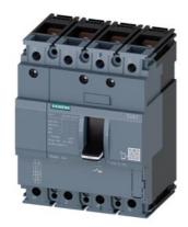
circuit breaker 3VA1 IEC Frame 100 breaking capacity class N Icu=25 kA @ 415 V 4-pole, line protection TM210, FTFM, In=25 A overload protection Ir=25 A permanently set short-circuit protection Ii=12.8 x In N conductor unprotected nut keeper kit
