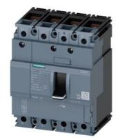
circuit breaker 3VA1 IEC Frame 100 breaking capacity class B Icu=16 kA @ 415 V 4-pole, line protection TM210, FTFM, ln=16 A overload protection lr=16 A permanently set short-circuit protection li=20 x In N conductor unprotected nut keeper kit
