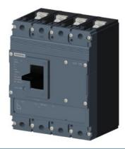
circuit breaker 3VJ1 IEC framesize 3VJ11 125A line protection FTFM 4-pole lcu=55kA@415V lcs=75% lcu In=20A overload protection Ir=20A short-circuit protection Ii=450A Screw connection
