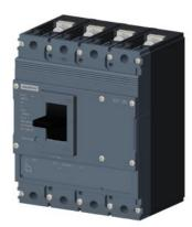
circuit breaker 3VJ1 IEC framesize 3VJ11 125A line protection FTFM 4-pole Icu=55kA@415V Ics=75% Icu In=100A overload protection Ir=100A short-circuit protection Ii=10 x In Screw connection
