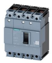
circuit breaker 3VM1 IEC frame 160 breaking capacity class S Icu=36kA @ 415V 4-pole, line protection TM210, FTFM, In=32A overload protection Ir=32A, not adjustable short-circuit protection Ii=10 x In N conductor protection 100% nut keeper kit
