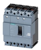
circuit breaker 3VM1 IEC frame 160 breaking capacity class S Icu=36kA @ 415V 4-pole, line protection TM210, FTFM, In=40A overload protection Ir=40A, not adjustable short-circuit protection Ii=10 x In N conductor protection 100% nut keeper kit
