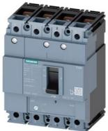
circuit breaker 3VM1 IEC frame 160 breaking capacity class N Icu=25kA @ 415V 4-pole, line protection TM220, ATFM, In=20A overload protection Ir=14A...20A short-circuit protection Ii=16 x In N conductor protection 100% nut keeper kit
