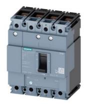
circuit breaker 3VM1 IEC frame 160 breaking capacity class N Icu=25kA @ 415V 4-pole, line protection TM220, ATFM, In=32A overload protection Ir=22A...32A short-circuit protection Ii=10 x In N conductor protection 100% nut keeper kit
